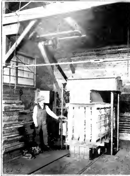
AUTOMATIC HYDRAULICALLY OPERATED DOOR VENEERING MACHINE INSTALLED IN PLANT OF COMMERCIAL SASH, DOOR & BLIND COMPANY, BEAVER FALLS, PA.
